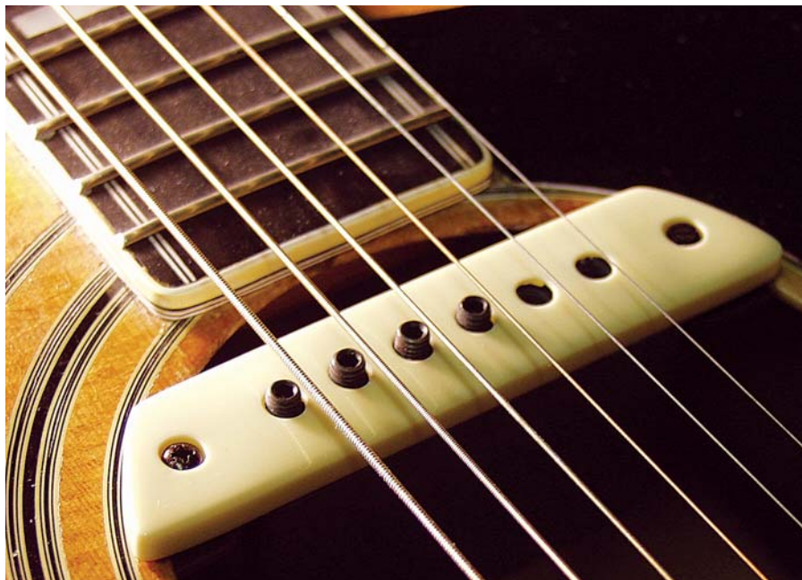
LR BAGGS’ M1 is a soundhole magnetic humbucker whose bottom coil, suspended to move freely below the main coil, functions as a dynamic body-sensing transducer. A new active version will debut at the 2005 winter NAMM show.
