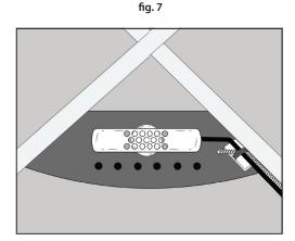
This is an internal view with the Tru • Mic mounted on the center of the bridge plate. The Tru • Mic and Element wires are secured with one wire clip on the bass-side of the bridge plate near the exit hole.
