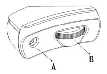
**A. MIC LEVEL CONTROL** (Adjusts the level of the Tru • Mic relative to the level of the Element)
