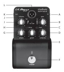
gain control in the counter-clockwise position. Turn the control clockwise as you play until the VU meter flashes yellow consistently. If red flashes too frequently, the input is clipping and you may experience unwanted distortion.
