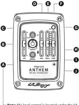
Note: Mic level control is located under the lid of the battery drawer. **A. Mic Level Control:** (Located under the lid of the battery drawer). Function: Sets the level of the Tru•Mic relative to the level of the Element pickup.
