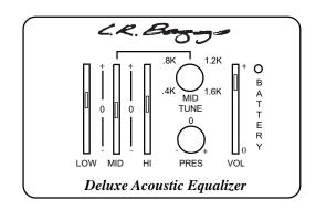
**Battery status LED:** Stays on when the unit is on and then flashes when the battery is low. The LED will start flashing when the battery reaches 6 volts. When it reaches 5 volts, it will stop flashing and fade away.
